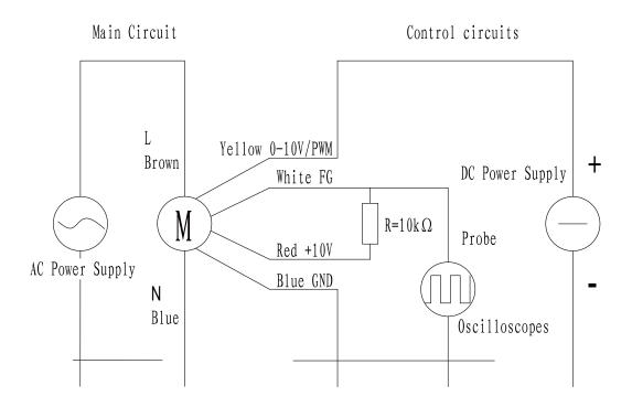
7-1. The fan has a speed output signal, and the waveform of the output signal is shown in the following figure. Vfg and pull-up resistor are external parts of the customer, Vfg=(3.3-30) VDC,  $R \ge 1000 \times (Vfg) \Omega$ .
