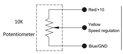
Suggest using a 10K potentiometer for speed regulation When the voltage is higher than 1.0VDC, the fan starts The fan stops when the voltage drops below 0.5VDC The starting voltage of the fan needs to be greater than 1.0V DC
