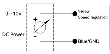
To use a DC power supply, it is necessary to support voltage regulation from 0~10VDC
