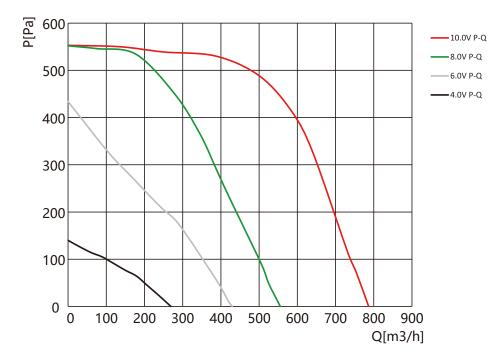
The air performance is measured according to AMCA210 and GB/T 1236. For detailed information on measurement settings, please contact us; The given values are valid under the specified measurement conditions and may vary due to installation conditions. For deviations from the standard configuration, the parameters must be checked on the installed equipment.
